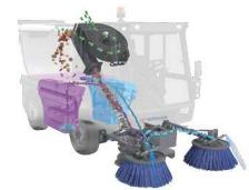
The 2-broom system with independently controlled circular brushes guarantees absolute mobility in every sweeping situation. Two stable broom arms with integrated buffers allow sweeping widths of up to 2,900 mm. Swingo 200<sup>+</sup> | 3-Brush
