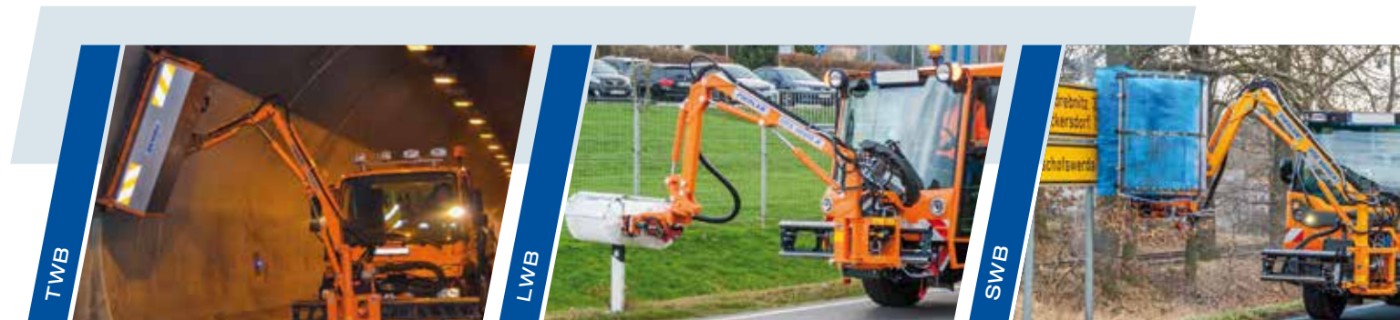
TWB – Tunnel washing brush | LWB – Marker Post washing brush | SWB – Sign washing brush
