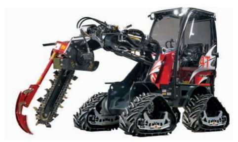
With the trencher you easily dig narrow trenches without damaging the ground in the digging area. It's a fast way to dig trenches for pipes or cables. The trencher does a clean trench which can easily be filled with a bucket or a blade. The trencher is driven by a hydraulic motor via a planetary drive to ensure a long and trouble-free operation.
