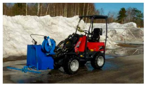
Equipped with a high-pressure washer it will turn you Norcar loader in to a smooth street cleaning machine. The washer handle and 20m of retractable hose makes it easy and efficient to wash your loader or other machinery and equipment. It is also suitable for washing benches, playgrounds, sidewalks, etc. The pressure washer combines low water consumption (301/min) with high pressure (200bar).
