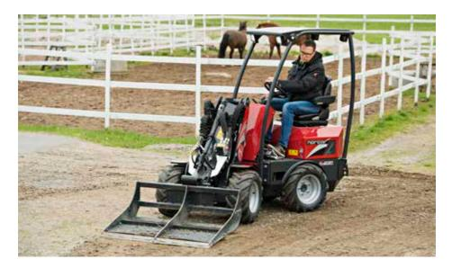
Landplane HD is an efficient and powerful attachment for grading and levelling before putting in lawns, gravel isles and preparing for brick isles and driveways. It grades, levels in both forward and reverse, peels and removes earth. It can even carry material like a bucket. The deluxe landplane includes a removable screen to pulverize soil lumps, aerate and sort debris from the soil.
