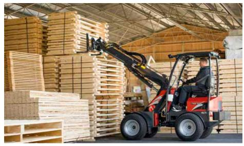
The forks are manufactured in high tensile forged steel. The adjustment of the forks is easy thanks to the quick lock mechanism. The pallet forks are suitable for lifting and handling of different types of materials on pallets.
