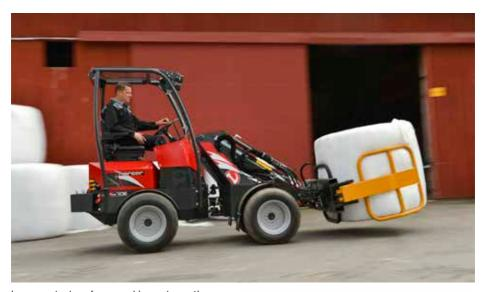
Large contact surfaces enable you to gently move plastic wrapped round bales. The grab handles round bales with a diameter from 99 cm to 180 cm. Powerful construction, steel blasted and treated with an alkyd paint that guarantees long durability and it's equipped with 2 powerful hydraulic cylinders 63/40-169 mm.
