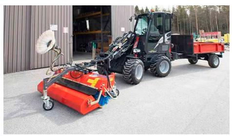
A versatile brush unit that can be equipped with a collector, a lateral brush and a water system.
