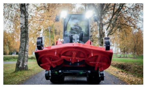
A stable hydraulically driven lawn mower with 3 belt driven rotors. The mover is a mulcher type and with a double cutting edge on each rotor the grass is spread out very effectively.
