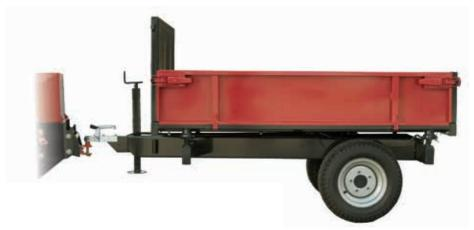
Powerful and versatile trailer with a 3-way tip. The direction of tipping is easily changed by moving the hinge pins placement. Equipped with foldable 35 cm high side walls that can be removed if necessary which opens a totally flat and even bed. The trailer has a very strong frame and a height adjustable trailer coupler.
