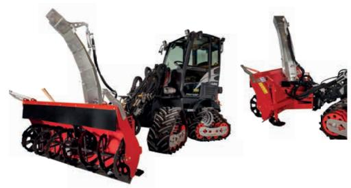
Norcar snow blowers are equipped with hydraulic controls for discharge chute rotation and throwing angle.
