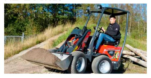
HD buckets are customized and designed for demanding use. The design and volume of the HD bucket is made to get a safe use even with heavy material on respective Norcar loader modell. Taking in consideration their tipping load value.
