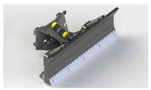
Effective tool for removing snow. Stable spring released mechanism with hydraulic turning. The blade has a floating system allowing the blade to float vertically, which makes working on uneven surfaces considerably easier and more efficient. The blade can be equipped with extensions. Comes standard with support plates and reversible wear plates (hardened steel AR500). Extensions 25+25 cm can be mounted in straight or collecting position (only on 8000262).
