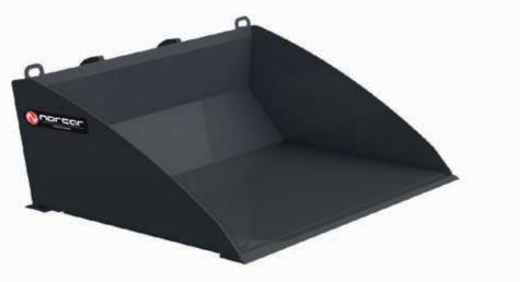
Heavy duty levelling bucket. Low rise design and a long bottom gives excellent visibility to the front edge of the bucket. The bucket has a 12 mm thick cutting edge in both the front and the rear which provides efficient levelling and cutting even in tougher materials.
