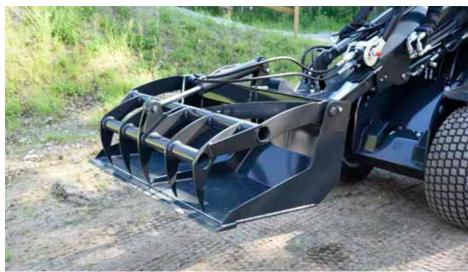
Grapple bucket is a combination of bucket and grapple. With the grapple bucket you can transport and load for example branches, wood chips, compost, bedding, manure and construction waste. With the grapple in the upper position it can also be used as a normal bucket.
