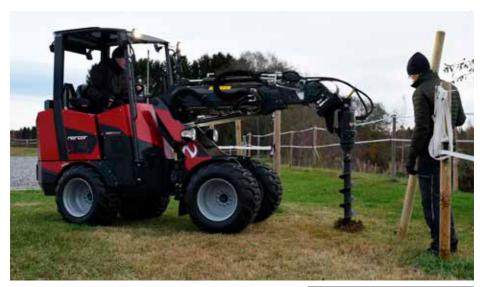
A hydraulic motor with a planetary drive gives you a high torque and makes the auger unit very efficient in many tasks. A large selection of different size augers makes it possible to drill holes from 75-900mm. To auger in hard ground conditions is made possible thanks to the replaceable tungsten teeth and pilot head.
