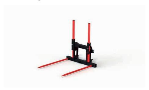
Sturdy attachment for handling both square and round bales. It has two high quality spring steel spears with a yield strength of over 1400 MPa. The spears are positioned so that they can also be used as a fork lift, which makes it very useful for handling both bales and pallet material without having to change anything. The attachment has height-adjustable support beams that protect against loads falling backwards.
