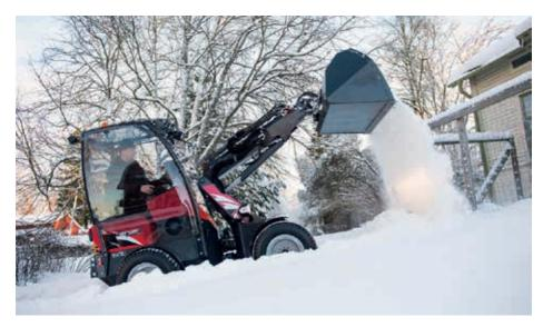
A bucket with great volume customized for lighter materials such as snow, soil, peat or wood chips. The buckets configuration with bent side plates and a draft angle towards the rear wall of the bucket guarantees a simple and complete emptying of the bucket with all kind of materials. The high upper edge of the bucket does that transported material doesn't fall backwards. The reinforced cutting edge on the bucket can handle very tough handling.
