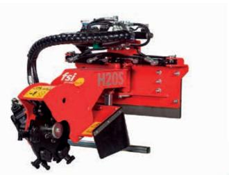
The stump grinder is mounted on the loader's attachment plate. The stump grinder has an integrated swing movement.
