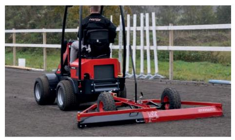
Effective tool for levelling and loosening horse arena riding surfaces. The graders blade can be opened and angled backwards and can then be used to move material from the arena walls to the center.
