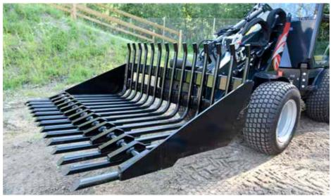
The stone collecting bucket is intended mainly for collecting stones from the fields after the field has been harrowed.
