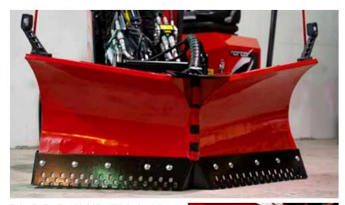
Hydraulically adjustable folding V-blade plough that facilitates snow removal along narrow sections. The folding of the plough is engaged easily and smoothly via the loader's joystick. The blade can also be turned horizontally (6°) in order to follow the surface in the best manner. The plough is equipped with corner markers. The hardened steel liner on the V-blade is replaceable. The hydraulic system is protected by an overpressure valve.
