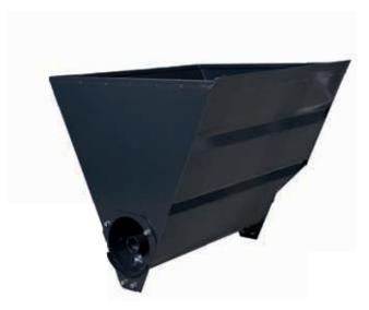
The dosing feeder is shaped like a bucket for easy filling of different materials. The auger in the bottom distributes the material smoothly and evenly. An attachment that is suitable for filling cable or pipe trenches. It can even be used for distributing animal feed. Suited for sand, finer gravel and flour.
