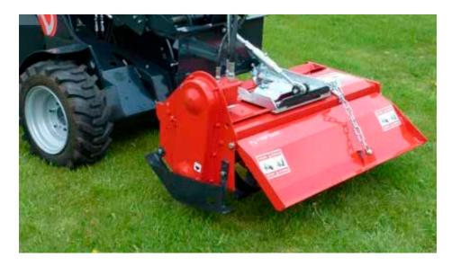
The rotary tiller has powerful rotors with 4 cutting blades each. The tiller cultivates the soil effectively. Very effective when making grass lawns and gardens.
