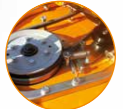
Engine crankshaft and bladeshaft are separated: Engine protection on impacts
